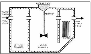
Aeration systems can purify waste water much more thoroughly than septic tanks. Sometimes they can remove as much as 90 percent of organic material and suspended solids. However, aeration systems have disadvantages too; they require servicing and maintenance more frequently than septic tanks. An aeration system uses electricity to operate the mixing mechanism and therefore is vulnerable to power failures. Aeration tanks are usually more expensive to purchase and install than septic tanks.
